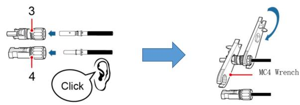
Step 2 Insert crimped PV positive and negative power cables into corresponding PV connectors
