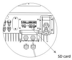
**Step 2** Press the SD card and take it out. Insert the SD card into a micro-SD card reader, then insert micro-SD card reader into a PC; (NOTE: micro-SD card reader & PC are not provided by SOFARSOLAR).
