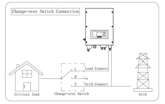
Fig. 15 Change-over Switch connections
