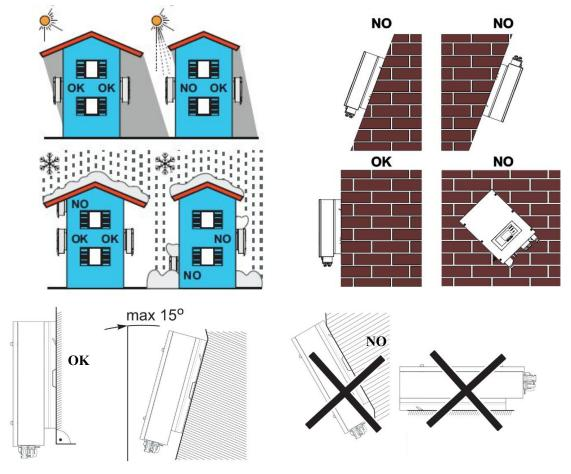
Fig. 4 Installation Position of HYD-ES inverter
