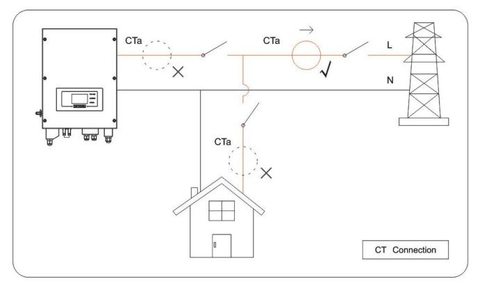
CT (Current transformer) can measure the value and direction of AC current. Refer to Fig. 11 for the correct connection of CTa.
