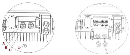
Fig. 12 CT / CAN / RS485 / NTC connection
