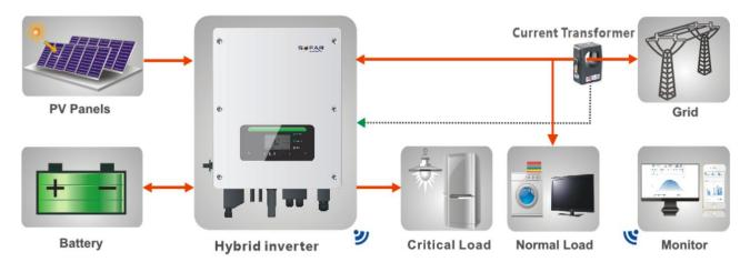
Fig. 1 HYD-ES inverter schematic diagram
